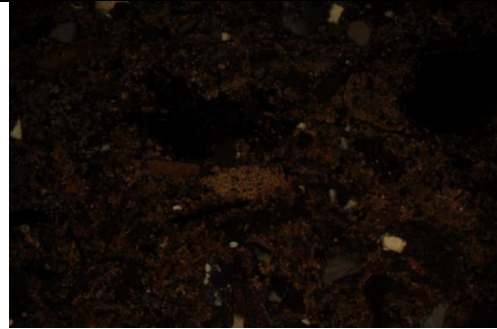
Fig. 24: As Fig 23, under XPL; the unweathered patch of ash (centre) has the highest birefringence.
